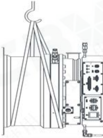
Figure15 Lifting schematic diagram (horizontal) (taking MTP-3201CTMS(ISO250F) as an example)
