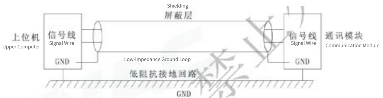
Figure 34 Grounding Example (Both Ends Grounded)
