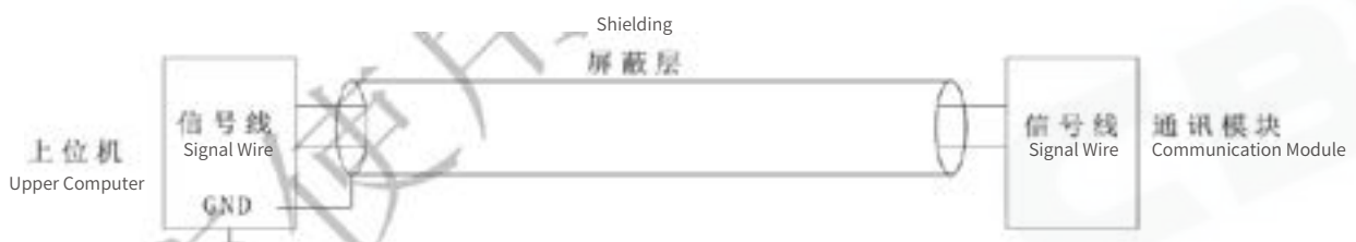
Figure 35 Grounding Example (Single-point Grounding)
